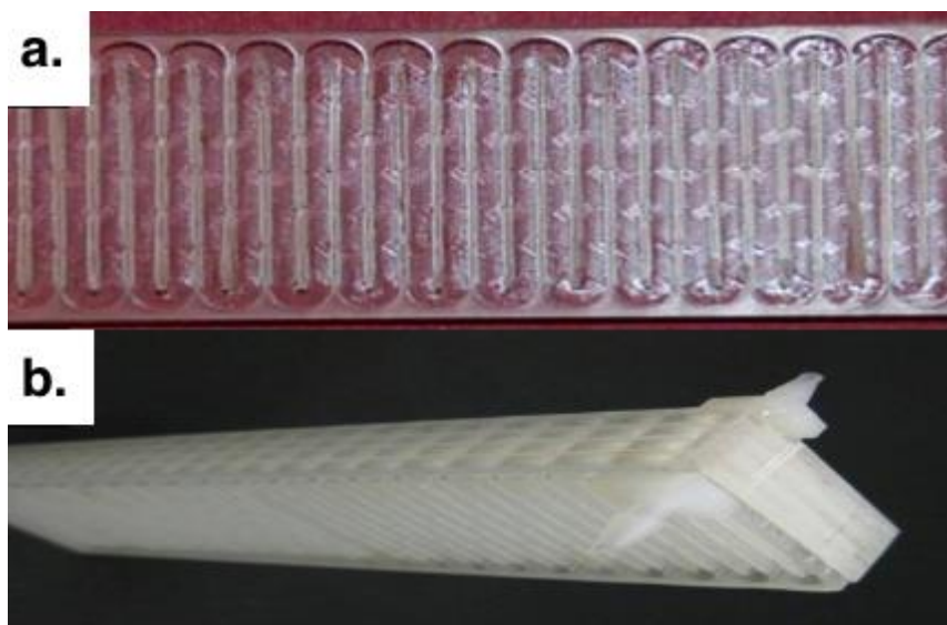
Figure 1. Fabricated microreactor module. a) Single fabricated cell b) reactor module built from single cells
