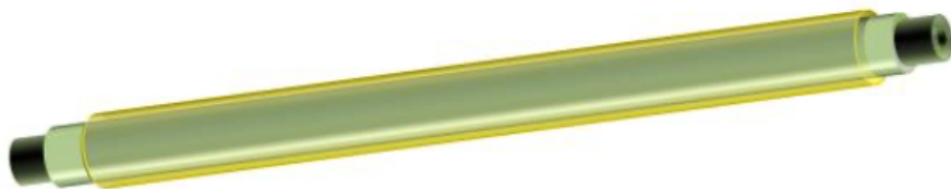
Figure 1. Schematic image of a 3D printed nitric oxide release polymer tube. Each layer contains a different nitric oxide concentration with darker layers representing a greater nitric oxide concentration from 2-5%. Devices printed range from a 1/16 of an inch diameter and greater.
